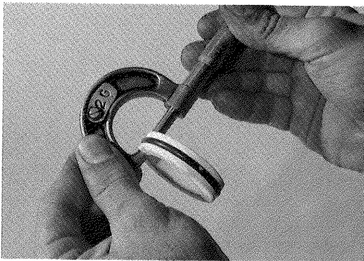
Figure 15—Carbon stationary face being checked for parallelism between sealing ring face and mounting face.
